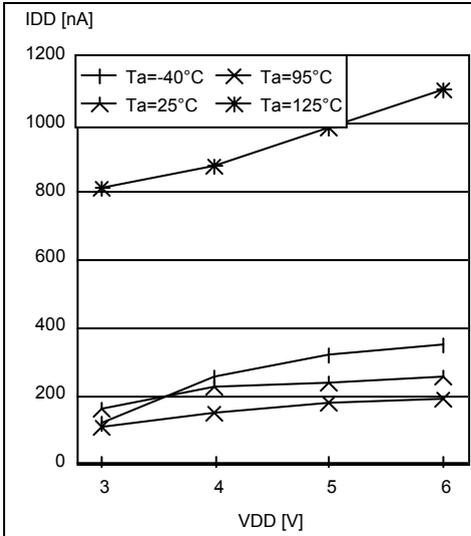
**Figure 42. Typical I<sub>DD</sub> in STOP vs Temperature for ROM devices**
