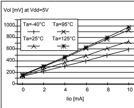
Figure 58. Typical  $V_{OL}$  at  $V_{DD} = 5V$  (high-sink)
