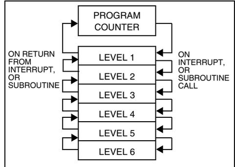
Since the accumulator, in common with all other data space registers, is not stored in this stack, management of these registers should be performed within the subroutine.
