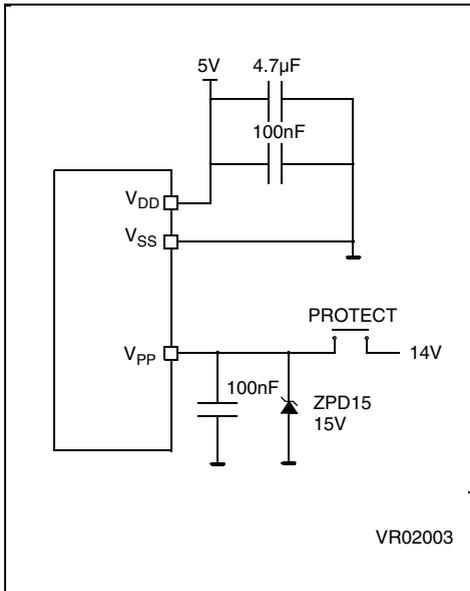
**Note:** ZPD15 is used for overvoltage protection
