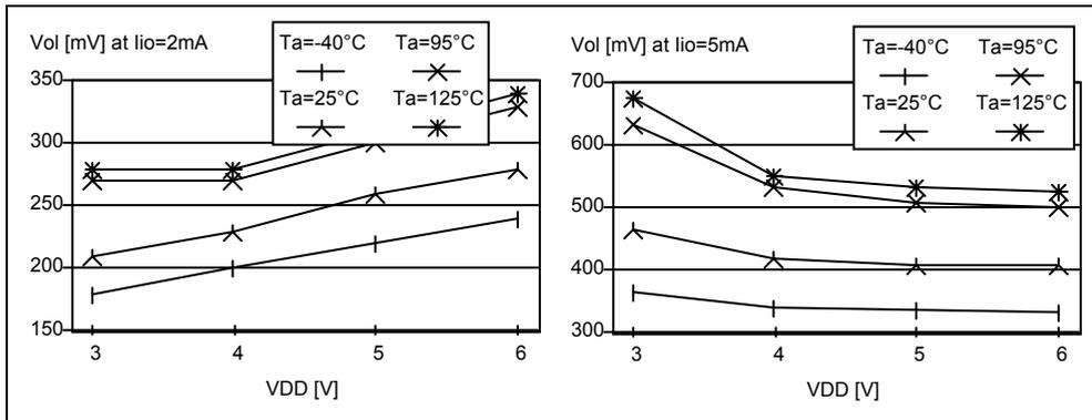
Figure 61. Typical  $V_{OL}$  vs  $V_{DD}$  (high-sink I/Os)
