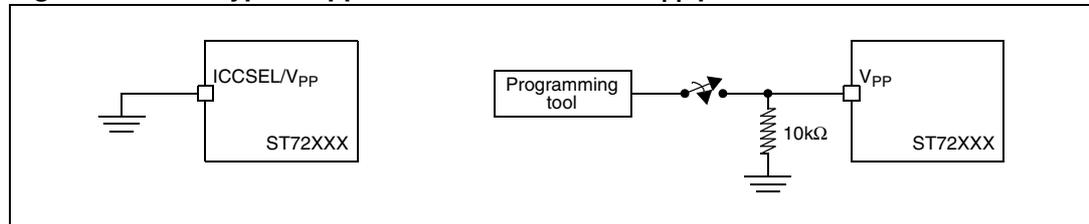
1. When ICC mode is not required by the application ICCSEL/V<sub>PP</sub> pin must be tied to V<sub>SS</sub>.
