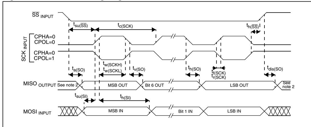
1. Measurement points are done at CMOS levels:  $0.3xV_{DD}$  and  $0.7xV_{DD}$ .
