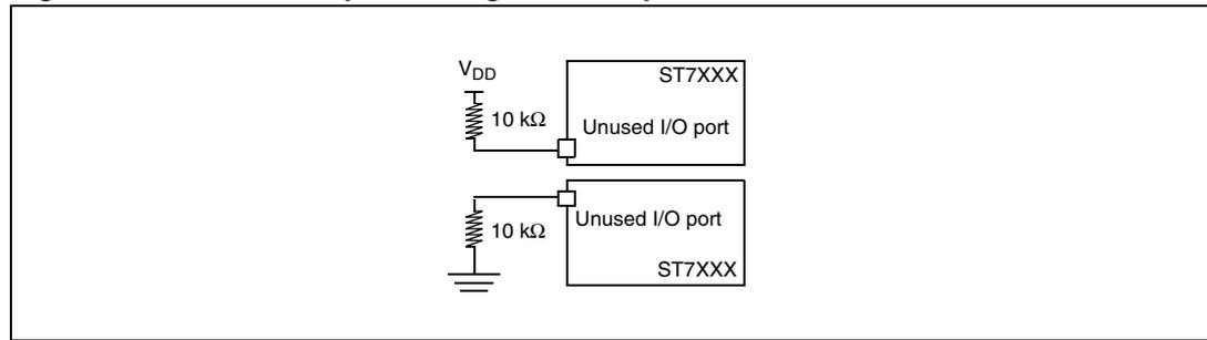
1. I/O can be left unconnected if it is configured as output (0 or 1) by the software. This has the advantage of greater EMC robustness and lower cost.
