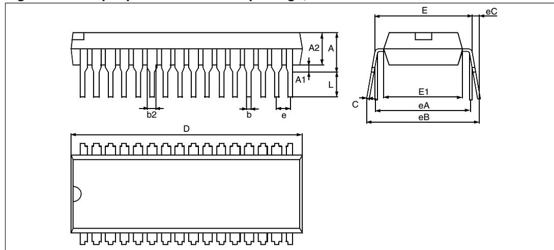
**Table 117. 32-pin dual in-line package mechanical data**
