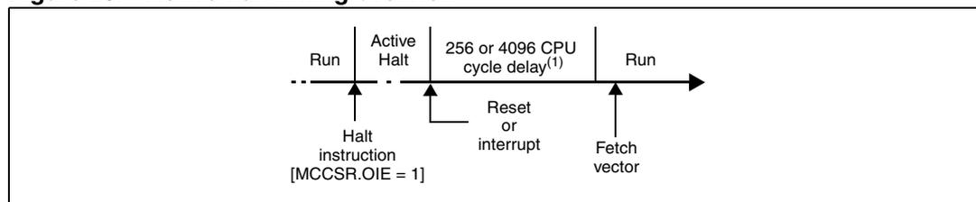
1. This delay occurs only if the MCU exits Active-halt mode by means of a reset.
