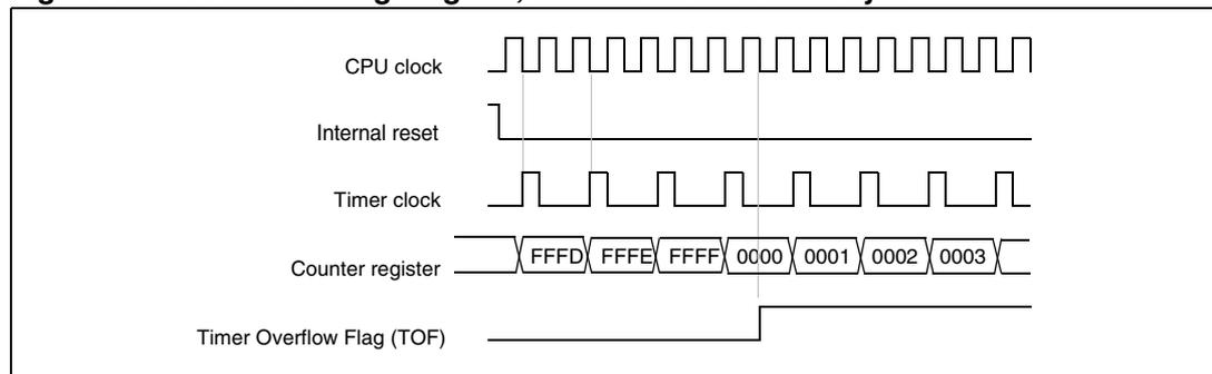
**Figure 39. Counter timing diagram, internal clock divided by 4**
