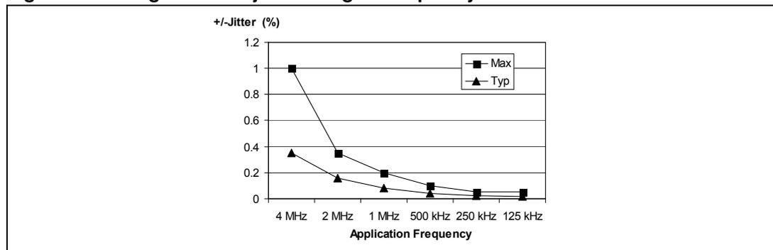
1. Measurement conditions:  $f_{CPU} = 8 \text{ MHz}$
