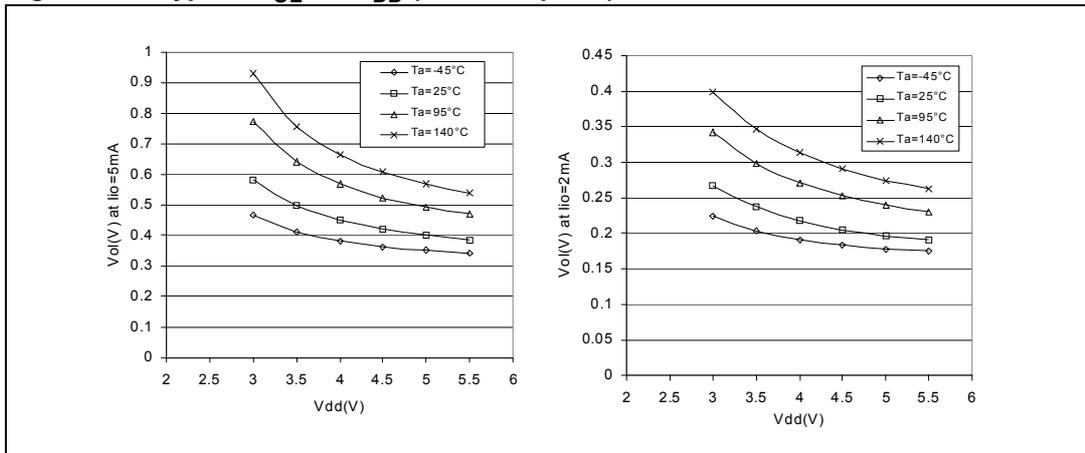
Figure 76. Typical  $V_{OL}$  vs.  $V_{DD}$  (high-sink ports)
