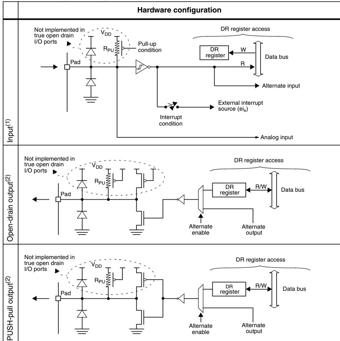
1. When the I/O port is in input configuration and the associated alternate function is enabled as an output, reading the DR register will read the alternate function output status.
