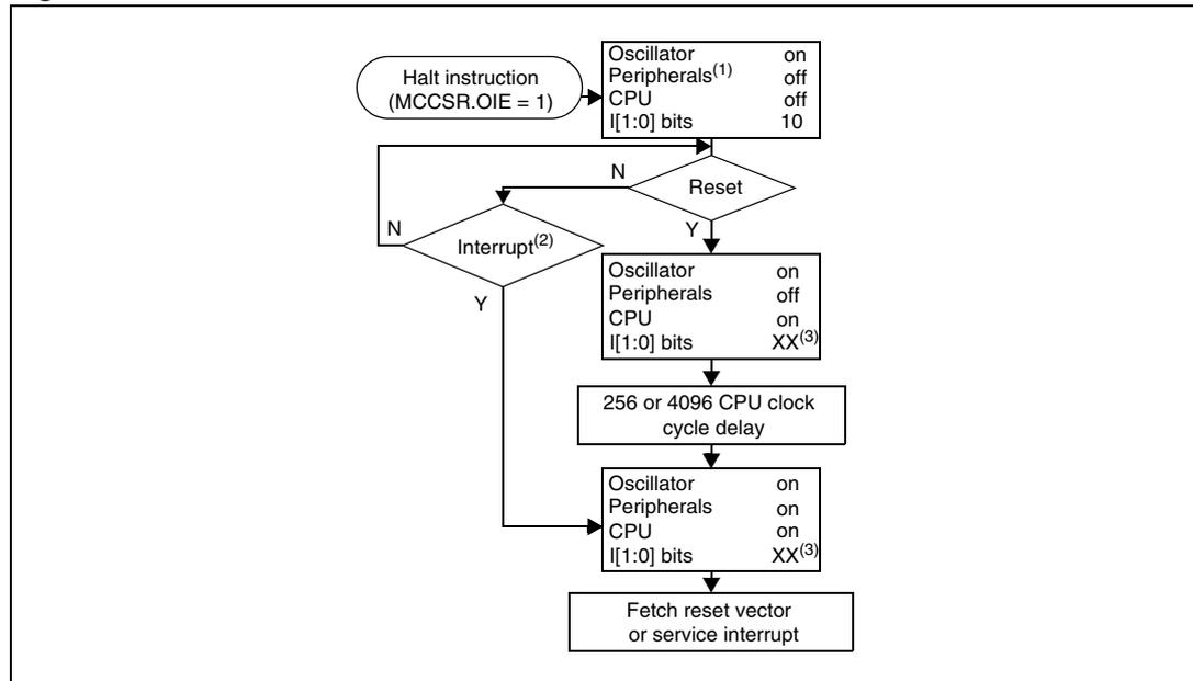
1. Peripheral clocked with an external clock source can still be active.
