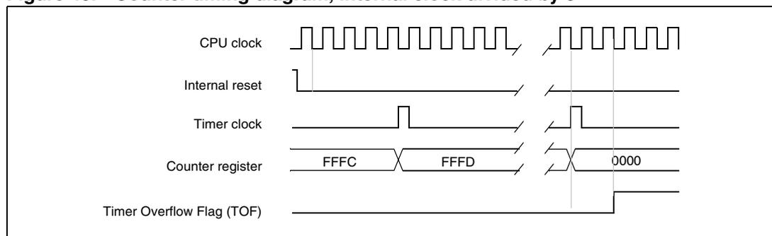
*Note:* The MCU is in reset state when the internal reset signal is high, when it is low the MCU is running.
