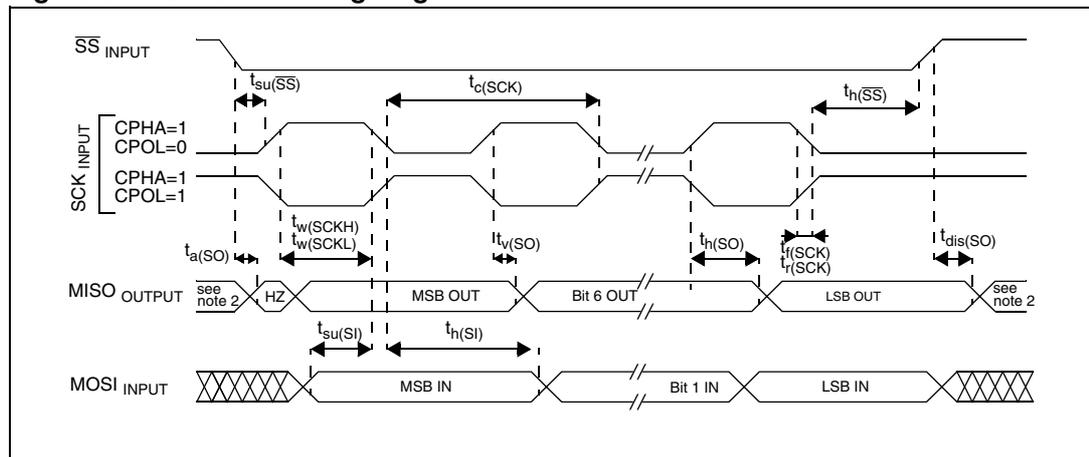
1. Measurement points are done at CMOS levels:  $0.3xV_{DD}$  and  $0.7xV_{DD}$ .
