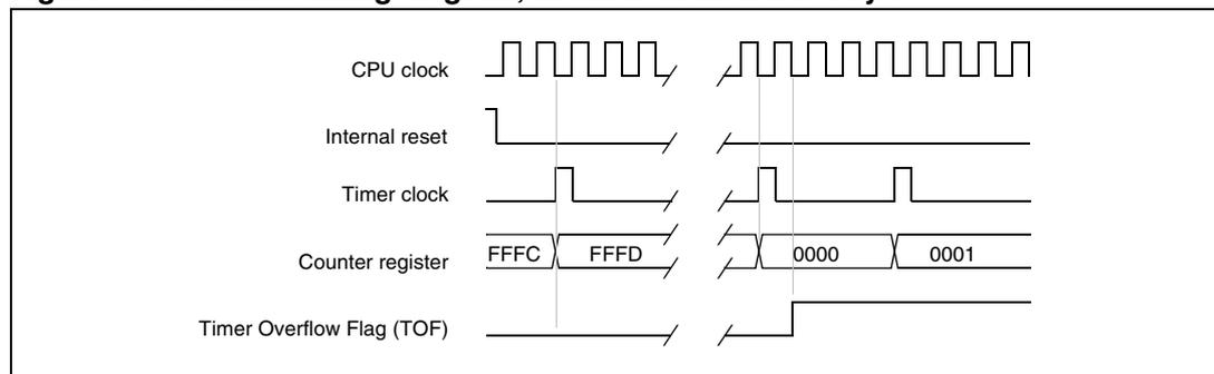
**Figure 40. Counter timing diagram, internal clock divided by 8**
