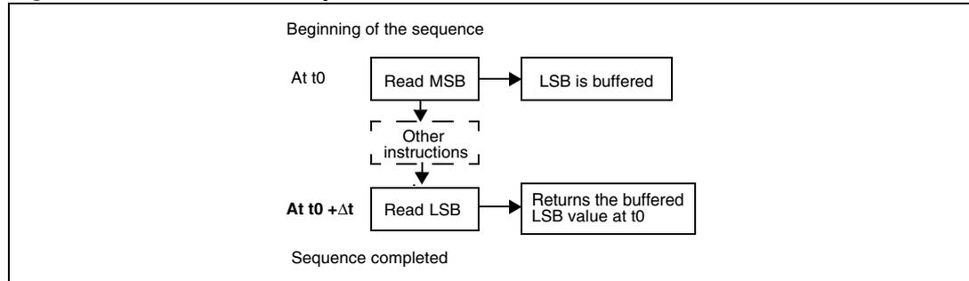
The user must first read the MSB, after which the LSB value is automatically buffered.
