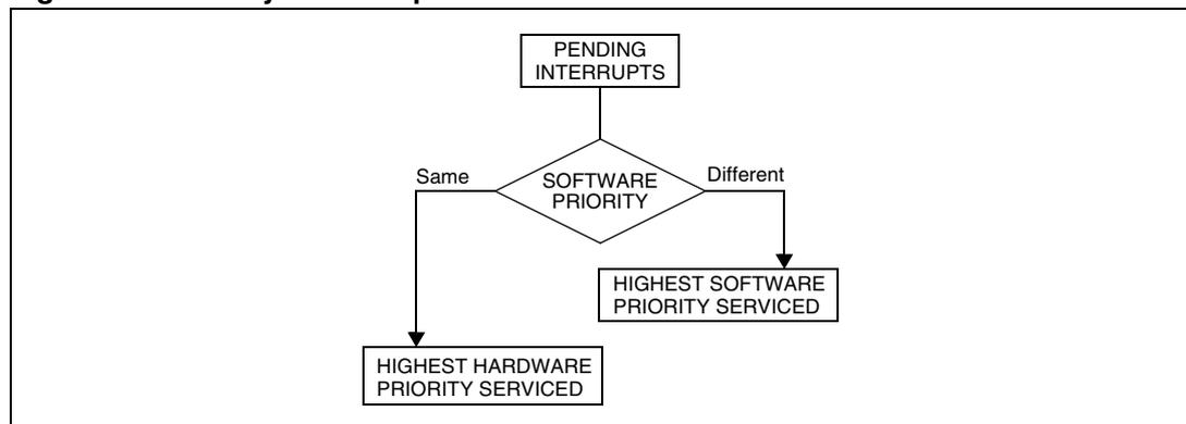
When an interrupt request is not serviced immediately, it is latched and then processed when its software priority combined with the hardware priority becomes the highest one.
