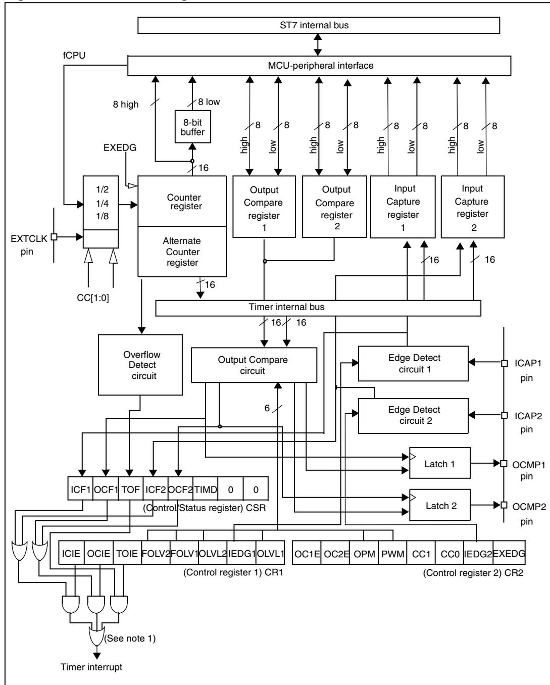
1. If IC, OC and TO interrupt requests have separate vectors then the last OR is not present (see [Table 25: Interrupt mapping on page 51](#)).
