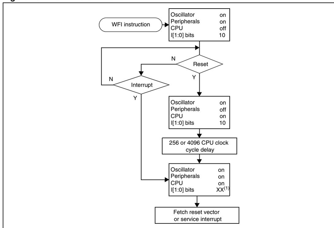
1. Before servicing an interrupt, the CC register is pushed on the stack. The I[1:0] bits of the CC register are set to the current software priority level of the interrupt routine and recovered when the CC register is popped.
