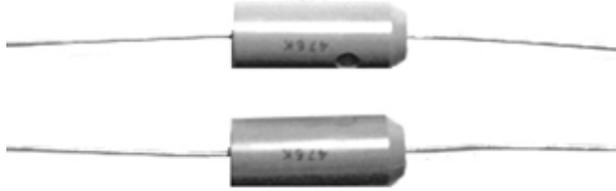
The Type TAC molded solid tantalum capacitor is great for putting a lot of capacitance in a small space in a high temperature application. The TAC is constructed in a shock and vibration resistant, flame retardant, rugged, precision molded case that is tapered on one end for polarity identification and available on tape and reel.
