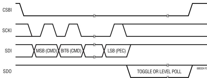
Figure 6. Transmission Format (PLADC Conversion or PLINT)
