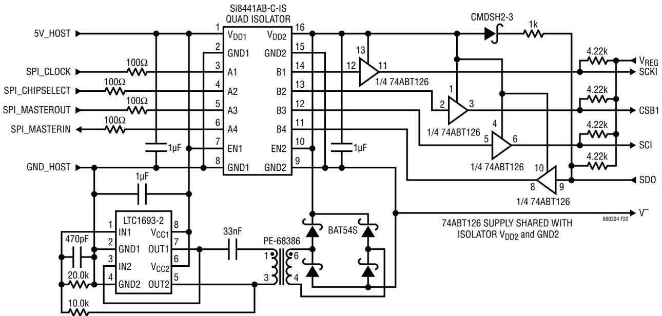
Figure 20. Providing an Isolated High Speed Data Interface
