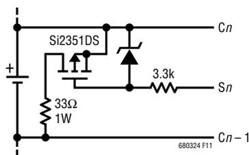
Figure 11. External Discharge FET Connection (One Cell Shown)
