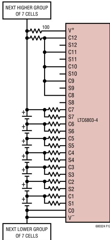
Figure 12. Monitoring 7 Cells with the LTC6803-4
