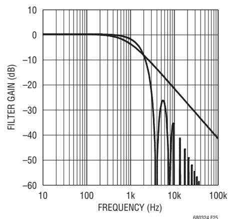
Figure 25. Noise Filtering of the LTC6803-4 ADC
