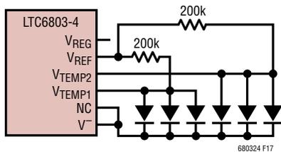
Figure 17. Using Diode Sensors as Hot Spot Detectors
