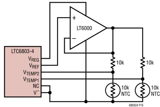
Figure 15. Buffering  $V_{REF}$  for Higher Current Sensors
