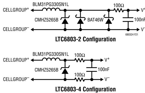
Figure 21. Supply Decoupling
