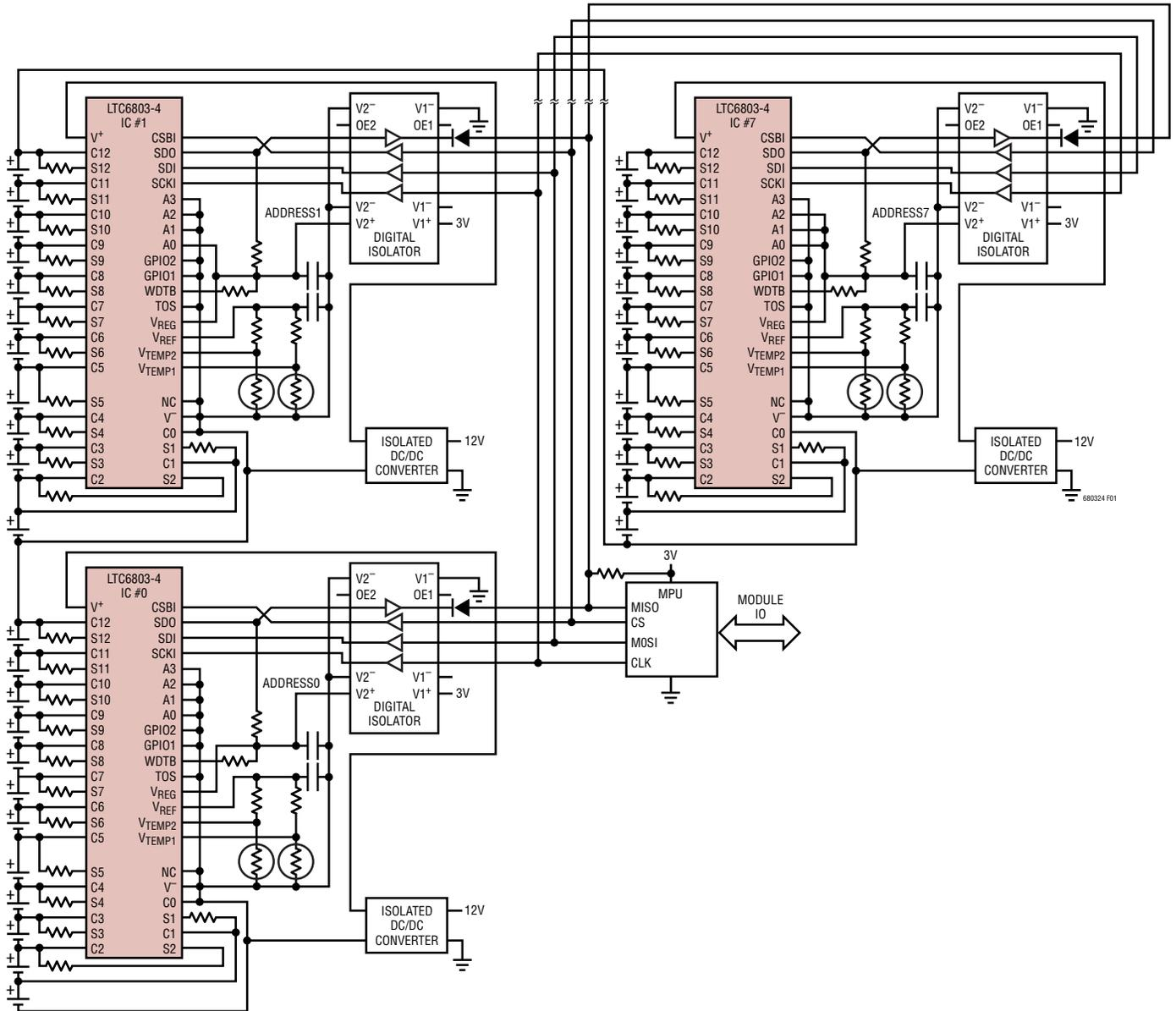
**Figure 1. Simplified 96-Cell Battery or Supercapacitor, Isolated Interface.** In this Diagram the Battery Negative is Isolated from the Module Ground. Isolated Power Supplies Each LTC6803-4. Opto-Couplers or Digital Isolators Allow Each IC to Be Addressed Individually
