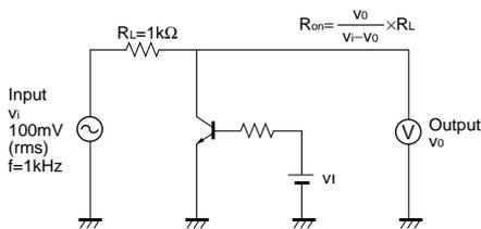
Fig.4 Output "ON" resistance (R<sub>on</sub>) measurement circuit
