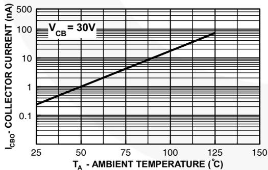
Figure 5. Collector Cut-Off Current vs. Ambient Temperature
