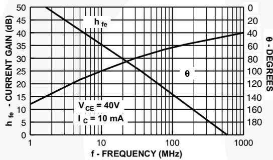
**Figure 9. Current Gain and Phase Angle vs. Frequency**
