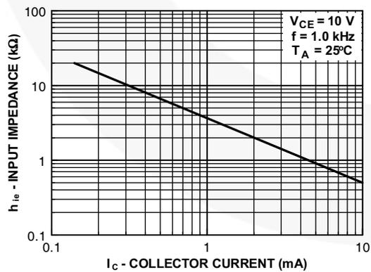
**Figure 17. Input Impedance**
