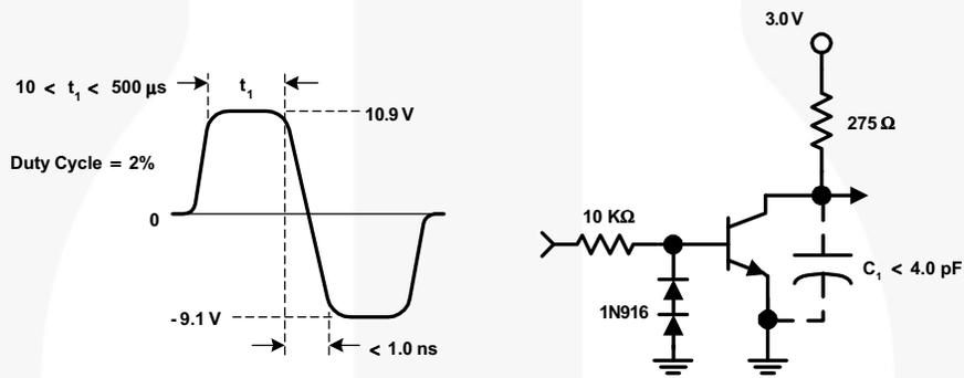
Figure 20. Storage and Fall Time Equivalent Test Circuit
