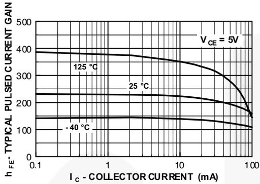
Figure 1. Typical Pulsed Current Gain vs. Collector Current
