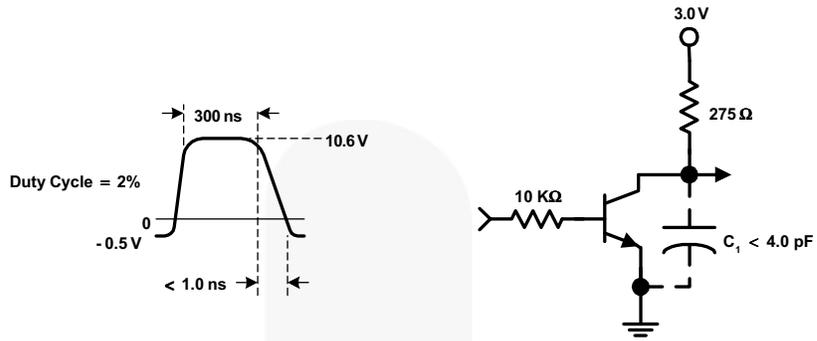
Figure 19. Delay and Rise Time Equivalent Test Circuit
